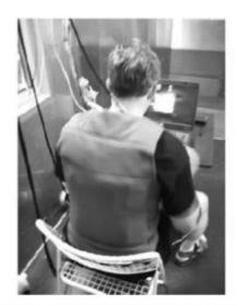
Fig. 2 A subject wearing the phase change materials (PCM) cooling vest on top of a T-shirt and instrumented with skin and rectal temperature sensors working with a personal computer at  $T_a=34^{\circ}\text{C}$ , RH=60%, and  $v_a=0.4$  m/s
